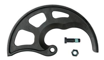
Replacement blade set for Klein's 63675 (2017 Edition) Cable Cutter. Hardened steel blades cut up to1000 MCM Copper and 1000 MCM Aluminum. Set includes moveable cutting blade, fulcrum screw, lock nut for fulcrum screw.
