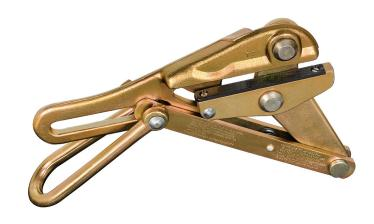
Designed for use on aluminum, copper, weatherproof coated wire, PVC covered conductors and messenger and guy strand. The Chicago style grip was designed for cable sizes from 0.16-Inch to 0.55-Inch (4.06 - 13.97 mm). Double V grooves give four-point contact, reducing chance of slipping and providing proper alignment of wire and cable.
