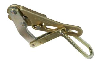
Designed for use on aluminum, copper, weatherproof coated wire, PVC covered conductors and messenger and guy strand. The Chicago style grip was designed for cable sizes from 0.218-Inch to 0.55-Inch (5.54 to 13.97 mm). When pulling EHS (extra-high-strength) galvanized-steel cable, the galvanizing has a tendency to coat the jaws of any grip, causing the cable to slip. Double V contour reduces the possibility of slippage and damage to the cable.
