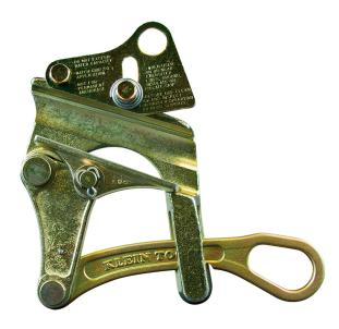
This parallel jaw grip was specifically designed to securely pull slippery HDPE-coated cable or tree wire. The innovative high-traction surface grips the cable without damaging the outer jacket. The tough carbide grit technology withstands even the harshest jobsite conditions. The grip is spring-loaded for one-handed operation and easy placement on the conductor.
