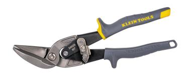
Cut and trim sheet metal in comfort with the Klein Tools straight cutting Offset Snips. Snip blades are made of forged, heat-treated steel for strength and durability. Offset blades make it easier to cut in tight curves and keep the user's hand away from the metal. The contoured plastic handles with thumb guards are color-coded by cutting pattern.
