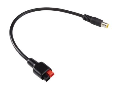
Klein Tools Anderson Powerpole®/APP® to DC cable with an 8mm Barrel Plug is compatible with Klein Tools Portable Power Station (Cat. No. KTB500) and Solar Panel (Cat. No. 29250). The 11.8-Inch flexible cord allows you to easily adapt your Solar Panel's APP® output to your portable power station's 8mm barrel plug charging input. Easily store the flexible cable in the pouch of Klein Tools Solar Panel.
