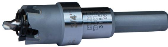
This carbide hole cutter cuts quick, precise holes in a variety of materials. Integrated flange prevents the operator from drilling beyond the sheet metal. Split point pilot drill bit prevents bit walking.
