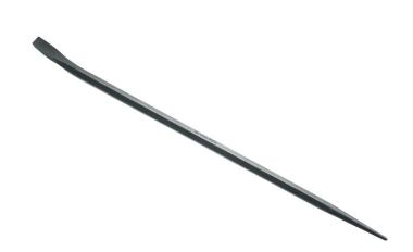
Klein Tools Hex Connecting Bars are designed so they provide extra-leverage when positioning steel members and aligning bolt holes. Hex bars are made of hardened steel for durability and long life. The chisel-end is at a 15-degree angle to give greater leverage.
