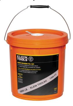
The Klein Tools 1800-Pound tensile strength conduit measuring pull tape is a durable, flat polyester strapping that disperses pull load and minimizes stretching when pulling. The tape is marked with descending 1-Foot increments to measure conduit runs. Tape is pre-lubricated to reduce friction and comes in a bucket with a hole in the lid for tangle-free dispensing. Pull Tape is also available in a variety of tensile strengths and lengths.
