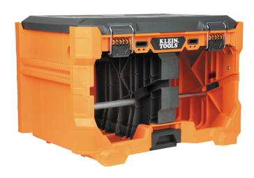
MODbox™ Wire Spool Dispenser streamlines wire management on the jobsite. It holds up to four 500-Foot spools of 10AWG wire inside and additional reels outside via a through-hole for conduit. Front guides and wire captures prevent unraveling. The lid with kickstand stays open for ceiling pulls. Built from impact-resistant polymers, supports up to 120 pounds, and has side rails for attachments. Easily connects with other MODbox™ components for a custom mobile workstation.
