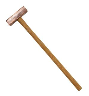
Klein Tools Copper Hammers are forged from pure electrolytic copper, so they are excellent for use in non-sparking environments. They can also be used to avoid damage to struck objects. This non-marking, soft-faced hammer does not contain oxygen, so unlike cast, it will not chip or break.
