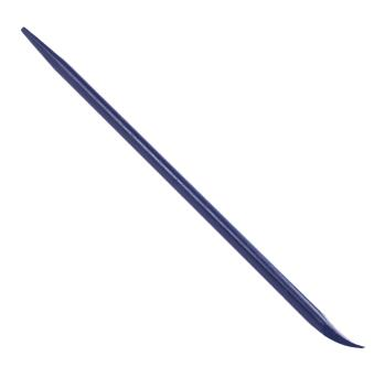
Klein Tools' Spoon Bars are excellent for levering, prying between surfaces and aligning holes. The taper is forged, not turned, which provides greater tensile strength. The thin spoon blade ends provide easy access between surfaces and a gentle rolling lift.
