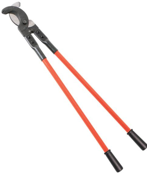
Klein Tools' Communication Cable Cutter is a lightweight, yet efficient shear-type cable cutter. It is designed to cut up to 900-pair soft copper and aluminum cable, and also lead or rubber-covered communications cable. Forged steel jaws make a clean, even cut for ease in fitting lugs and terminals.
