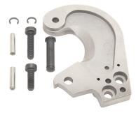
Replacement blade set for use with Klein's Cat. No. 63607 Ratcheting Cable Cutter (Pre-2017 Edition). Forged, heat-treated, shear-type cutting blades are made of hardened steel for sharpness and long life. Cuts up to 336 MCM ACSR, 400 MCM copper and 600 MCM aluminum.
