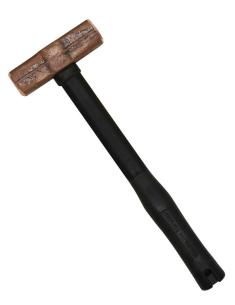
Klein Tools Copper Hammers are specially designed for use in non-sparking environments or to avoid damage to struck objects. The head is forged from pure electrolytic copper, which contains no oxygen, so unlike cast it will not chip or break. The comfortable thick rubber grip provides better protection from shock and vibration.
