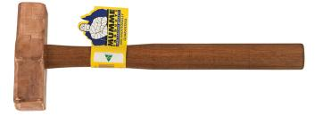
Klein Tools Copper Hammers are specially designed for use in non-sparking environments or to avoid damage to struck objects. The head is forged from pure electrolytic copper, which contains no oxygen, so unlike cast it will not chip or break. These hammers are fitted with a tough Australian spotted gun hardwood handle, which is oiled for long life and user comfort.
