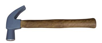
Klein Tools Normalized Claw Hammers are great for general woodworking applications, especially where risk of chipping and damage to struck objects need to be minimized. The head is forged from tough high-tensile carbon manganese steel. The face is normalized to be softer and less likely to chip.
