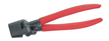
Use these Klein Tools Straight Seamer Tongs for working with sheet metal and HVAC materials. The tongs have padded handles and depth indicators marked in 1/4-Inch increments for precise bending.
