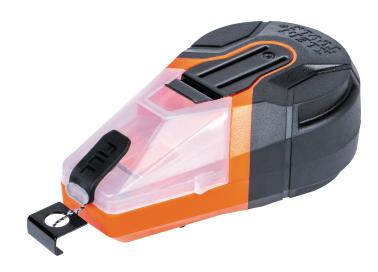
Klein Tools' 100-Foot Quick-Fill Chalk Line features jam-resistant gears, ensuring seamless retraction of the 100-Foot braided nylon thread. The 4 times faster 4:1 gear ratio surpasses traditional alternatives. Enjoy dual functionality as a chalk line and plumb bob for precise horizontal and vertical layouts. Transparent, refillable chalk capsules offer easy visibility and optimal refilling with Cat. Nos. CHLK14B, CHLK14R. The high-impact ABS case with soft grips guarantees lasting durability.
