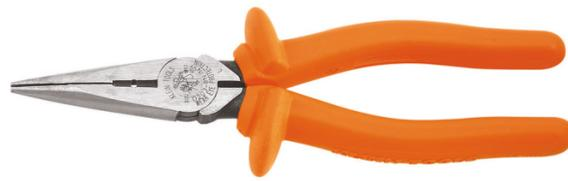
These Klein Tools long nose side-cutting/stripping pliers are made of forged steel for maximum durability. They have a heavier design and extended handles to improve leverage and power. And they have two layer bright orange insulation that is both flame retardant and provide electric protection for up to 1000 V.
