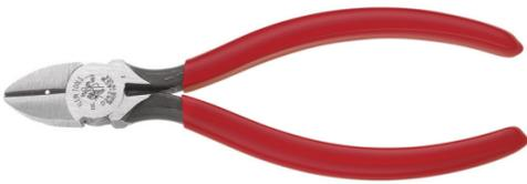
These Klein Tools Diagonal-Cutting Pliers Bell System have a heavier design for all purpose use. The pliers' bell system type has a skinning hole for 24 AWG and "W" notches slit insulation cleanly. They are made of US-made steel with induction hardened cutting knives for durability. The hot-riveted joint ensures smooth action and no handle wobble.
