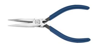
These slim long-nose pliers are great for extremely close-quarter work. The longer nose and handles provide a deeper reach. The polished inside jaws help prevent nicking of wires and are spring-loaded for self-opening.
