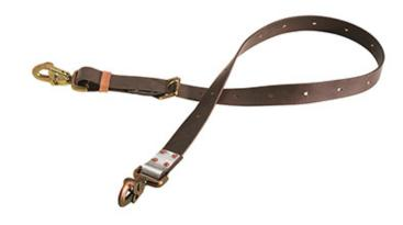
Klein's positioning straps work with Klein's climbing equipment for linemen. Made with exceptionally strong and long-lasting Klein-Kord, the straps are adjustable within a 2-Foot 3-Inch range. The drop-forged, single tongue adjustment buckle has a corrosion-resistant finish. Depending on the application, choose a positioning strap that allows you to work at arm's length from the pole or other positioning anchorage.
