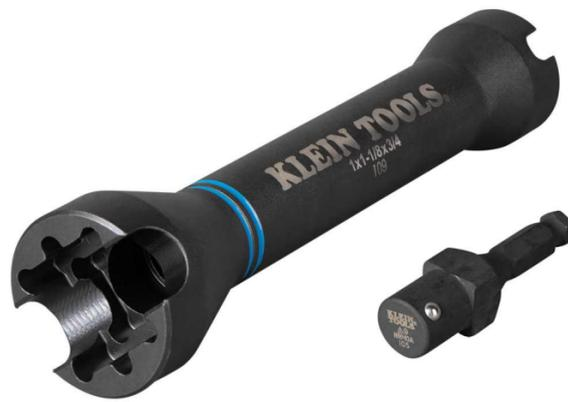
The Klein Tools versatile 5-in-1 Impact Socket reigns as the market leader for Linemen and Utility Workers. It features three popular square sizes that can be quickly and easily converted for a variety of utility type applications. Designed with an alignment slot to tighten and loosen most pole hardware. It also has a long, hollow shaft designed to fit over long threaded bolts.
