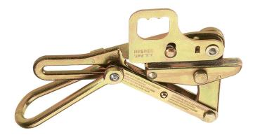
The Klein S1684-5H Chicago Grip-with Hot-Line Latch for Bare Conductors are for both bare and insulated conductors. The Klein S1684-5H Chicago Grip-with Hot-Line Latch for Bare Conductors grip may be placed on wire with hot-line stick. When stick is removed, latch closes automatically to guard against grip accidentally disengaging from wire.
