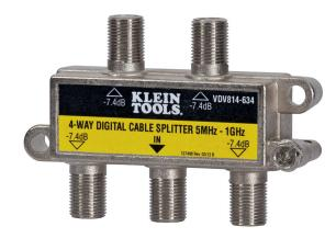
Klein splitters have lower insertion loss, higher shielding, a solder back cover and are hand-tuned for quality and performance. The Klein 4-Way Splitter is optimized for digital and high-definition connections. It splits signals for up to four outlets. Bandwidth specifications are 5 MHz - 1 GHz.
